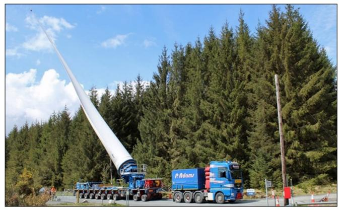
To undertake the transfer between trailers, a blade transfer area will need to be constructed. The area of land required will need to be circa 175m x 60m and will need to include two crane pads. Storage for up to six blades should also be available, with all infrastructure designed in accordance with turbine supplier standards.
